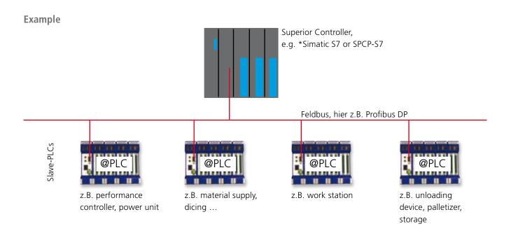
The @PLC acts the same way to a control system as a slave to a fieldbus. Therefore, it does not matter what programming language you use to program your controller. You have all the I/O modules to your disposal because we enter the same hardware like in the traditional fieldbus modules and of course with the full modularity of the @ctivelO system.
