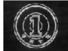
Sample Edge Detection Using a 1-Yen Coin
